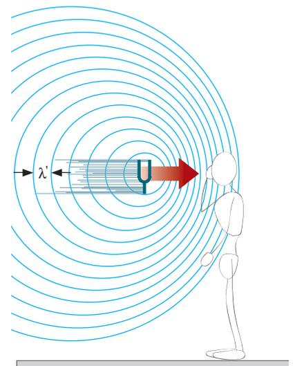
**Figure 16-13** If the source of sound moves toward the right, the waves bunch up on the right-hand side and spread out on the left-hand side. The person hears a frequency that is higher than that emitted by the source.
