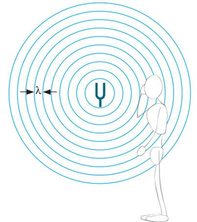
**Figure 16-12** If the source and the ear are stationary relative to each other, the ear hears the same frequency as emitted by the source.
